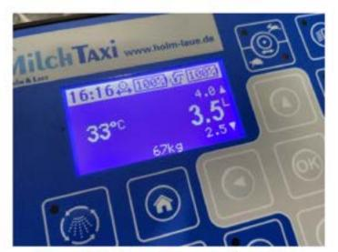
Smart-Mix only requires the desired milk replacer concentration and scoop size once. It then specifies the water quantity and weight of powder.
